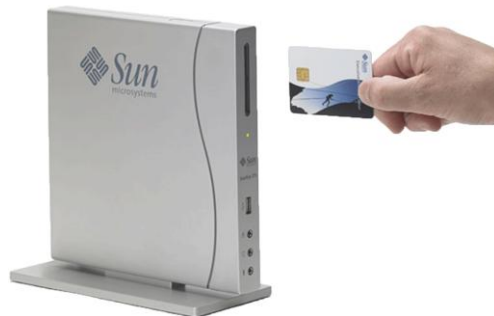
Figure 3 Inserting a smart card into a Sun Ray thin client
